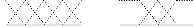
FIG. 2.1. The nodal bases of the spaces Z_k^l and \widetilde{W}_k^l ; here, the dimension of Z_k^l is five.
